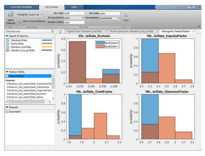
Control the appearance of the histograms using the parameters in the **Histogram** tab, which activates when you generate the histograms. The CrestFactor feature appears to separate healthy and unhealthy data almost completely. Investigate whether this result is sensitive to resolution. In the **Histogram** tab, the auto setting of bin width results in a resolution of 0.1 for CrestFactor. Enter a bin width 0.05, and click **Apply**.
