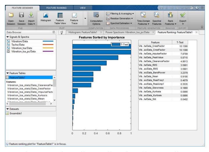
The app operates on data ensembles. An *ensemble* is a collection of data sets, created by measuring or simulating a system under varying conditions. An individual data set representing one system under one set of conditions is a *member*. **Diagnostic Feature Designer** processes all ensemble members when executing one operation.
